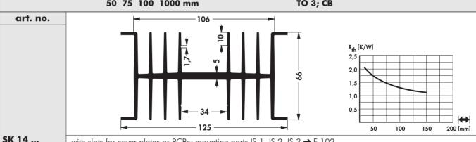
SK 14 ... with slots for cover plates or PCBs; mounting parts IS 1, IS 2, IS 3 → E 102
