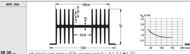
with slots for cover plates or PCBs; mounting parts IS 1, IS 2, IS 3 → E 102 please indicate: ... � (optional)
