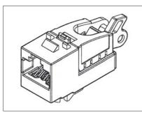
SPECIFICATIONS Dieletric Withstanging Voltage: 1000 V Insulation Resistance: 500 MΩ DC Current Rating: 1.5 Amps DC Resistance: 0.1Ω Contact Resistance: 20 mΩ Temperature Range: -10°C~60°C Insertion Life: 750 mating cycles with FCC compliant RJ-45 plug Contact Compatibility: Accommodates 23-24 AWG Solid
