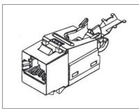
SPECIFICATIONS Dieletric Withstanging Voltage: 1000 V Insulation Resistance: 500 MΩ DC Current Rating: 1.5 Amps DC Resistance: 0.1Ω Contact Resistance: 20 mΩ Temperature Range: -10°C~60°C Insertion Life: 750 mating cycles with FCC compliant RJ-45 plug Contact Compatibility: Accommodates 23-24 AWG Solid
