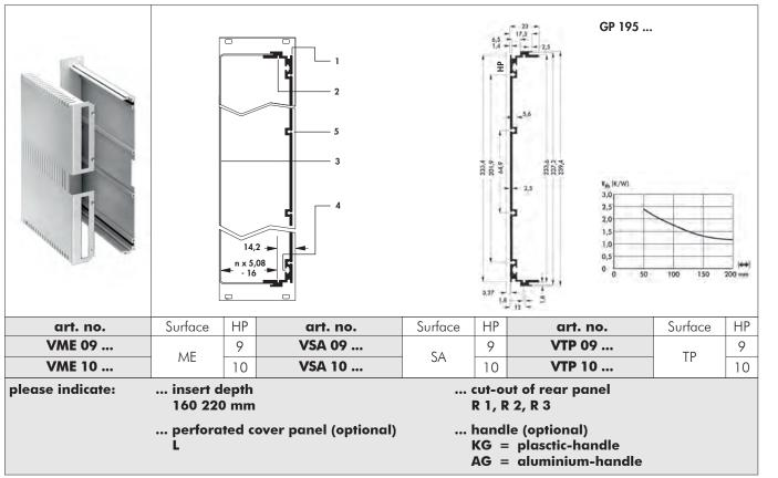
**ME** = front panel, profiles and rear panel natural colour anodised
