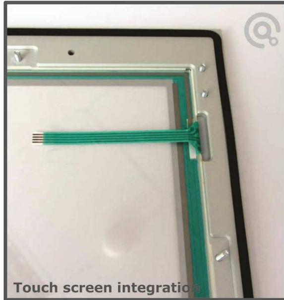
Also larger size of touch screens can be integrated with optical clear adhesives on graphic foil. Such panels can be used also in very demanded environment: medicine application, food production and similar. Panels where touch screens are protected with polyester foil offer perfect cleaning possibilities and suitable protection of application.
