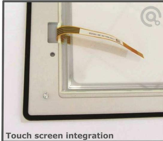
Complete front panel (exclusive touch screen) can be produced in our production. On pictures above we show Al panel, natural eloxated with inserted press-in-bolts and integrated gasket. Resistive touch screen is integrated with optical clear adhesive on antiglare polyester foil where graphic design was printed before. In final part of production process front foil was laminated on AL frame and touch screens was sealed with suitable resin.
