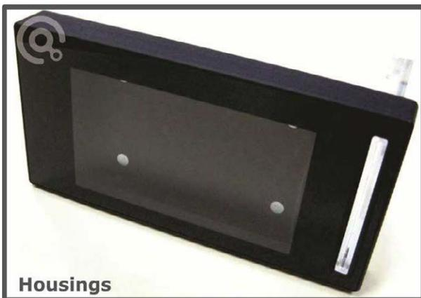
Aluminum housing, black eloxation, front side with hard-coated PMMA, printed color and integration of capacitive touch-screen, transparent illuminated card holder, Press-in-bolts for fixing on product housing.
