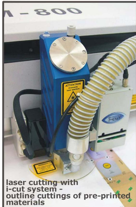
**laser cutting with i-cut system - outline cuttings of pre-printed materials**
