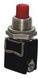
PBS-13B OFF-(ON) PBS-13C ON-(OFF) 4A 250VAC
