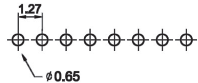
Recommended P.C.Board Layout
