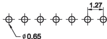
Recommended P.C.Board Layout
