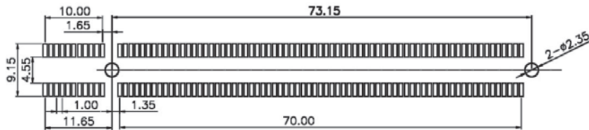
Recommended P.C.Board Layout (Top View)
