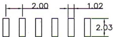
Recommended P.C.Board Layout
