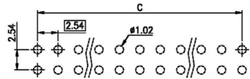
Recommended P.C.Board Layout
