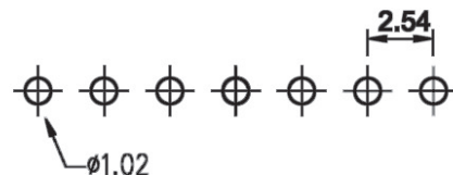
Recommended P.C.Board Layout
