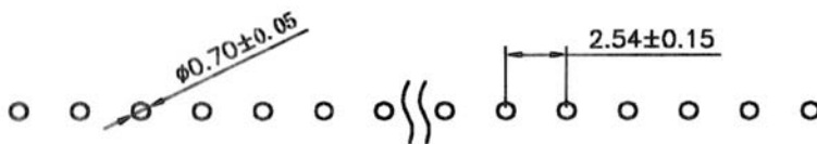
Recommended P.C.Board Layout
