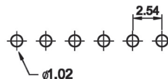
Recommended P.C.Board Layout
