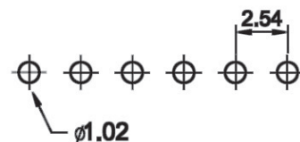
Recommended P.C.Board Layout
