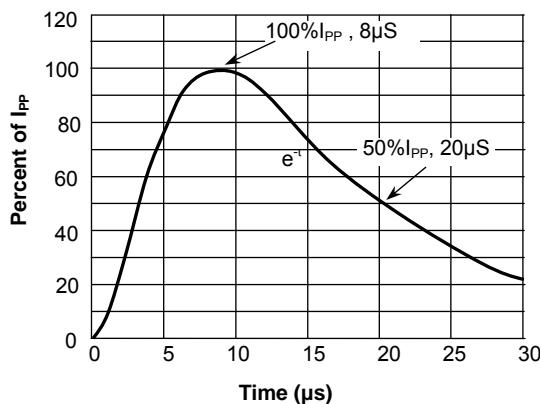
**Fig.4 Pulse Waveform-ESD(IEC61000-4-2)**
