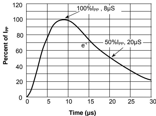
**Fig.4 Pulse Waveform-ESD(IEC61000-4-2)**
