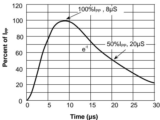
**Fig.4 Pulse Waveform-ESD(IEC61000-4-2)**
