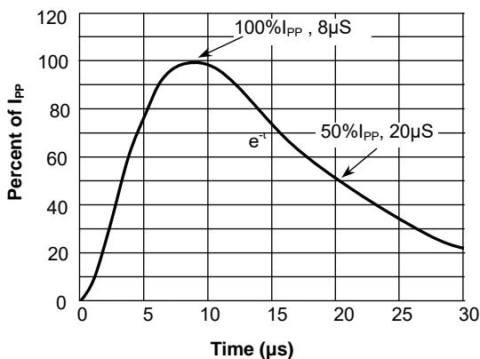
**Fig.4 Pulse Waveform-ESD(IEC61000-4-2)**
