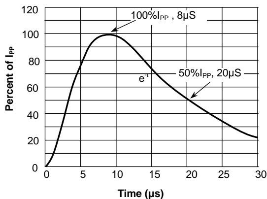
**Fig.4 Pulse Waveform-ESD(IEC61000-4-2)**
