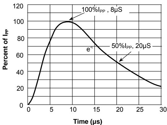
**Fig.4 Pulse Waveform-ESD(IEC61000-4-2)**
