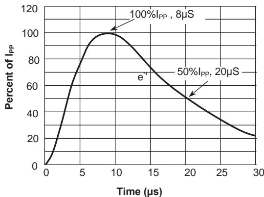
**Fig.4 Pulse Waveform-ESD(IEC61000-4-2)**
