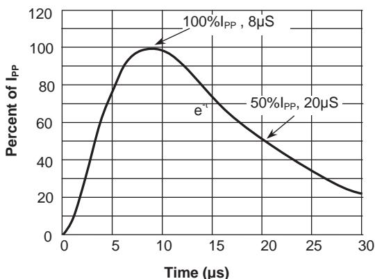
**Fig.4 Pulse Waveform-ESD(IEC61000-4-2)**
