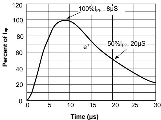
**Fig.4 Pulse Waveform-ESD(IEC61000-4-2)**
