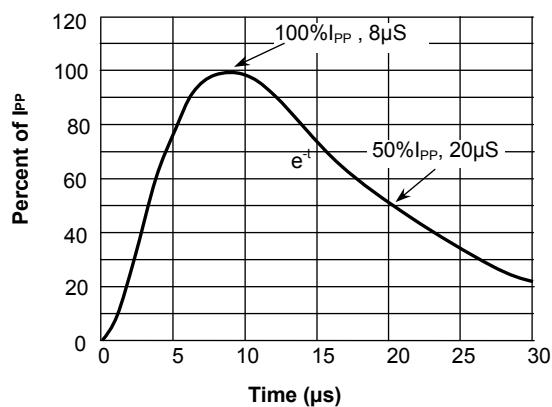
**Fig.4 Pulse Waveform-ESD(IEC61000-4-2)**
