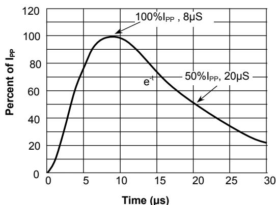
**Fig.4 Pulse Waveform-ESD(IEC61000-4-2)**
