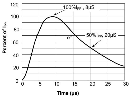
**Fig.4 Pulse Waveform-ESD(IEC61000-4-2)**
