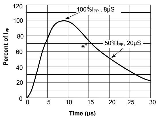
**Fig.4 Pulse Waveform-ESD(IEC61000-4-2)**
