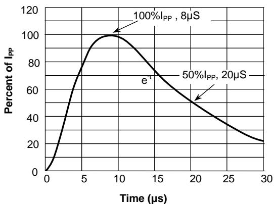
**Fig.4 Pulse Waveform-ESD(IEC61000-4-2)**
