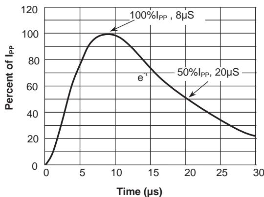
**Fig.4 Pulse Waveform-ESD(IEC61000-4-2)**
