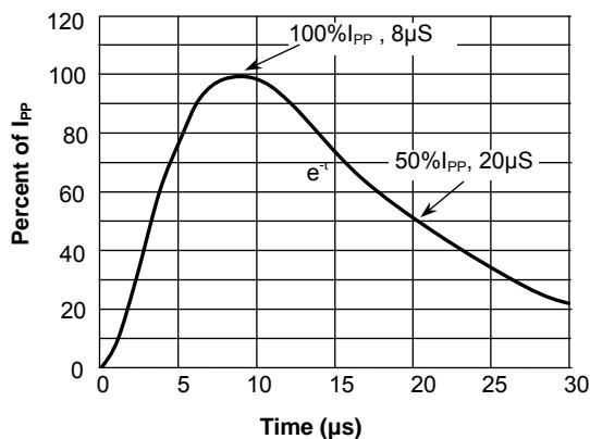
**Fig.4 Pulse Waveform-ESD(IEC61000-4-2)**
