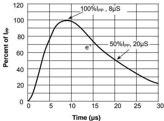
**Fig.4 Pulse Waveform-ESD(IEC61000-4-2)**
