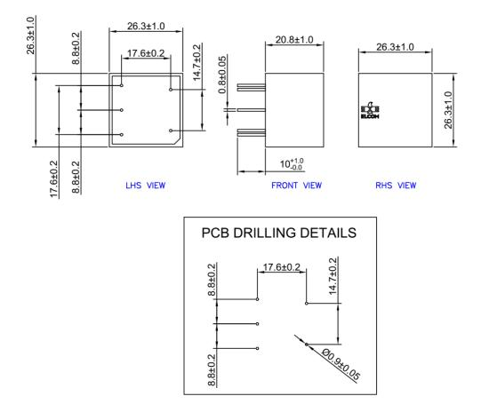
\*All dimensions are in mm. Note: For medical application filter, earthing terminal is not provided.
